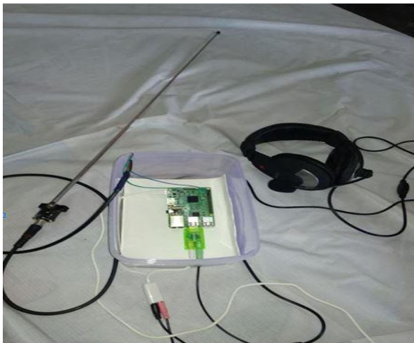
Fig10. Raspberry Pi transmitting voice signals
