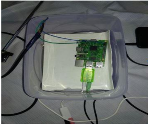
Fig9. Raspberry working as FM transmitter
